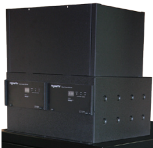
Chimney Duct, Fan Chassis, Fan Cartridges, on top of Cabinet
