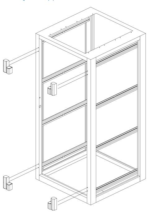
Step 1: Attach the "L" shaped portion of the hinge to the outside of the cabinet frame using supplied #10-32 Screws. (see diagram)
