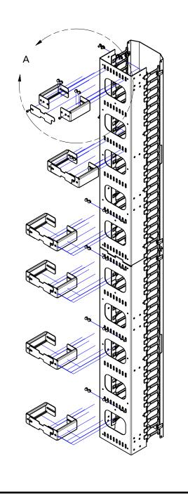
\* High density cable ring kits mount to the back of any cable managers (RFM-RHDV-XX-XX-SB) ranging from 6" to 10" max.
